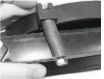
3. Install the Nylock nut and snug the nut. Install all 4 nuts and bolts before tightening. Tighten the nuts evenly until there is a slight pressure on all of the rubber spacers. Do not over tighten the nuts and Allen bolts, this will break the fan assembly.
