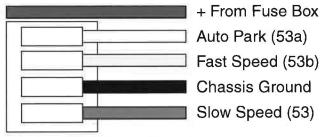
To be used with steering column mounted style switches only
