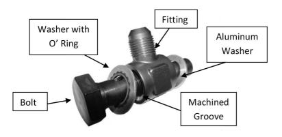
Bolt, Washer w/ O' Ring, Fitting with Machined Groove toward the O' Ring Washer, lastly the aluminum washer (between fitting and case). Clock the fitting to desired position then torque to 30lbs.
