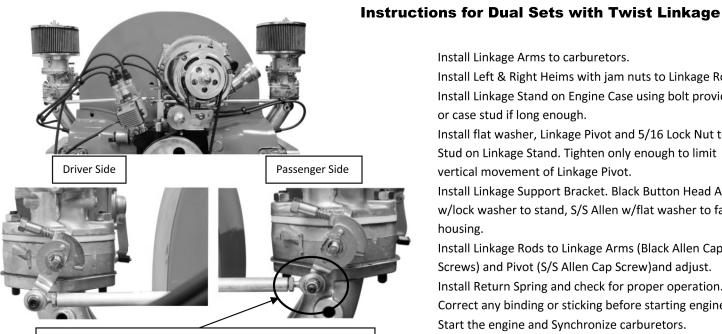
Right & Left Linkage Arms are the interchangeable. Passenger Side bolt must be installed from Inside - Nut on Outside
