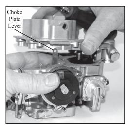
6. After changing the jets, be sure to install the top gasket and start the choke plate lever into the slot before reinstalling the mounting screws.
