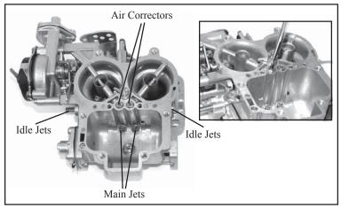
4. The air corrector jets are on the top of the carburetor over the float bowl. 99-4307/0106
