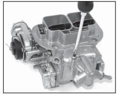
2. Remove the 6 mounting screws from the top of the carburetor and remove the top. Be careful not to tear the gasket.
