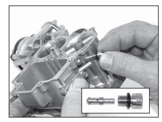
7. If changing idle jets, remove the jet and o-ring from the side carburetor (again the primary jet is over the butterfly with the throttle lever on it). Separate the jet from the holder by pulling them apart. Replace with new jet and reinstall. Be sure to push the o-ring back against the screw head.
