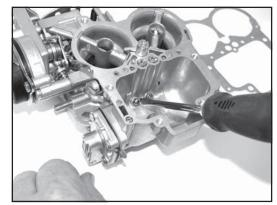
5. The main jets are located at the base of the float bowl. On a 32/36 progressive carburetor, the primary jets are over the butterfly with the throttle lever connected to it. If you are working on a 38 carburetor, both butterflies open at the same time so there is not a primary and both jets are the same size.
