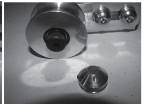
10. Remove billet cover from the idler pulley by loosening the set screw with a #2 allen wrench.
