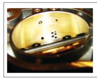
5-6 Progression Ports that allow for extremely smooth acceleration and drivability. Designed to bolt-on and run!
