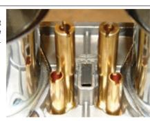
Decompression Valve – eliminates drips caused by pent-up pressure.
