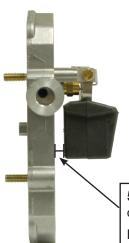
Float Setting is critical for proper fuel delivery. While the Floats have been set at the Factory, bouncing around in the back of a series of delivery trucks can often alter the adjustment. It is always best to check. While there, check and clean the float bowl for any debris. Remove the Carburetor Top carefully – the gasket is reusable if not torn during dis-assembly.
