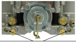
Air By-Pass Screws should remain closed.
