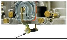
The Accelerator Pump Rod is set at the factory. It is not recommended to adjust the action of the rod to increase fuel delivery.
