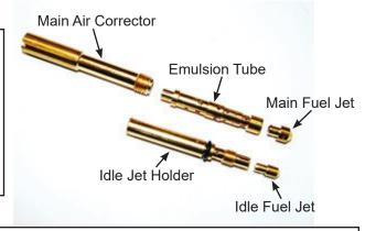
NOTE: Dirty and/or plugged Idle and Main Jets will lead to poor performance. If one or more cylinders are not firing properly – this is the first place to inspect and clean.
