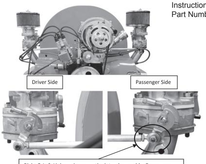
Right & Left Linkage Arms are the interchangeable. Passenger Side bolt must be installed from Inside – Nut on Outside
